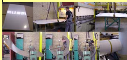
Figure 8: From plate to tube. The two tubes are for the load lock (cross tube).
